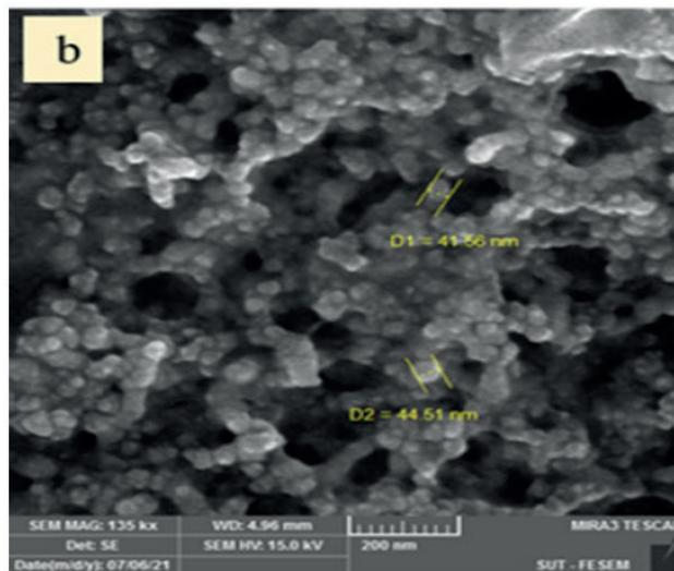
**Figure 5.** This is a figure of a Scanning Electron Microscopy image of AgNPs fabricated by *Microbacterium sp.* with a 41-44 nm diameter.
