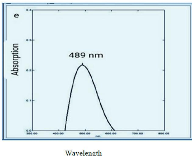
**Figure 2.** This figure of UV-Vis spectroscopy of AgNPs showed a peak at 489nm wavelength.
