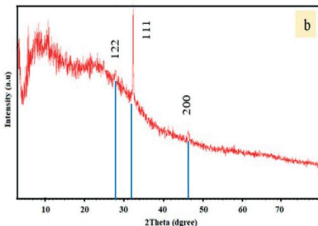
**Figure 3.** This figure of X-ray diffraction of synthesized AgNPs analysis, diffraction standards (JCPDS), silver file No. (04-0783).
