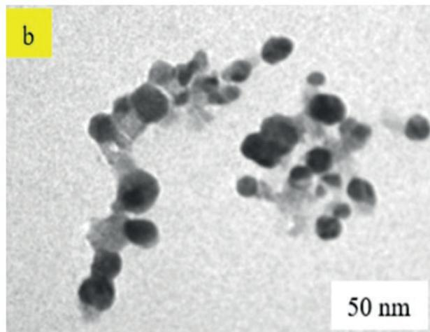
**Figure 4.** This figure of Transmission Electron Microscopy image showed the size of silver nanoparticle with an average diameter of around 50 nm.
