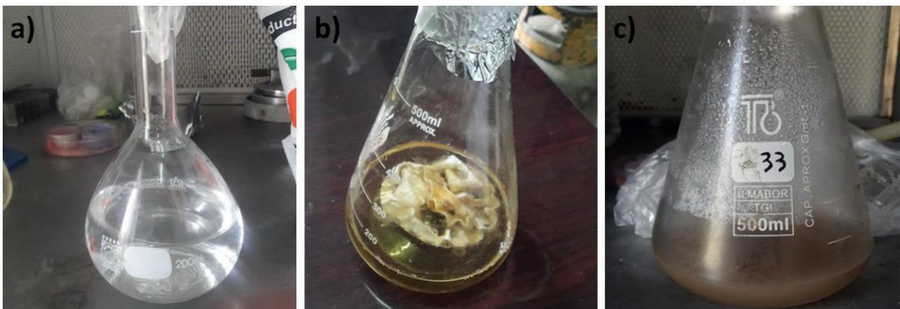
**Figure 2.** Synthesis of AgNPs: a) AgNO<sub>3</sub> (1 mM) solution; b) *A. terreus* biomass (50 mL); c) Color alteration of filtrate after incubation in the dark.
