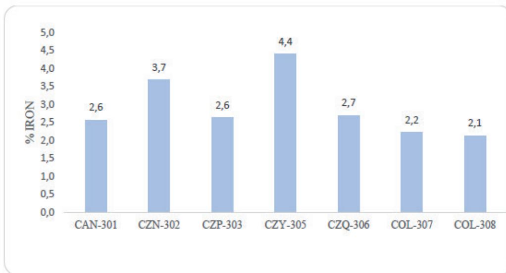
Figure 6. Percentage of iron concentration in clay samples obtained by Atomic Absorption Spectroscopy.
