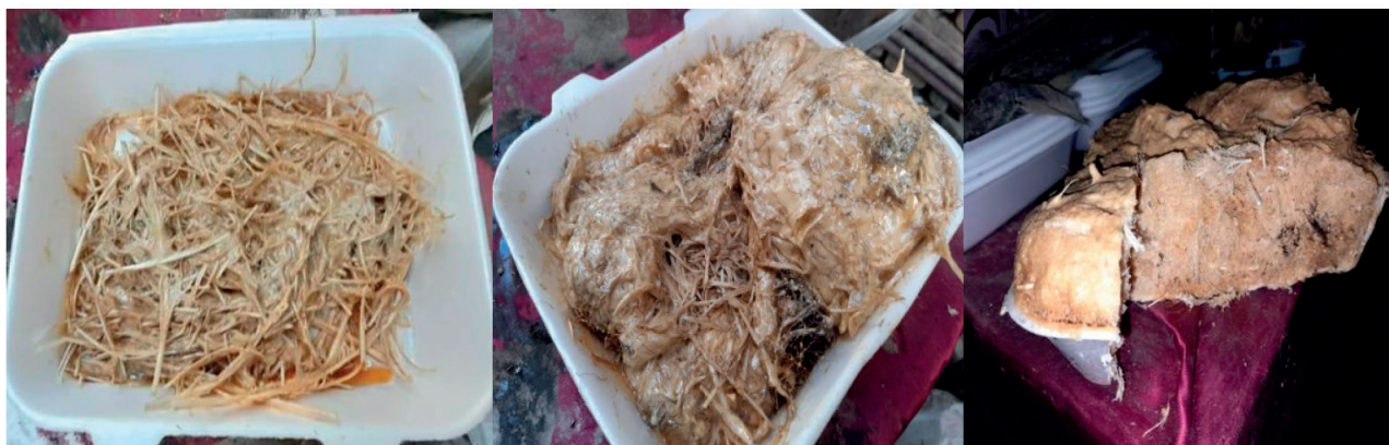
Figure 1. Shows the modified polyurethane foam added with feathers.
