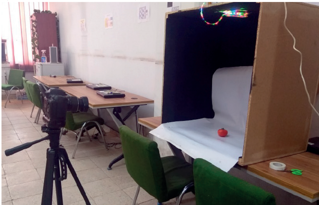
Figure 1. Studio for photos, Tomatoes and five replications, three pictures of the identical fruit were taken from the highest, bottom and side.
