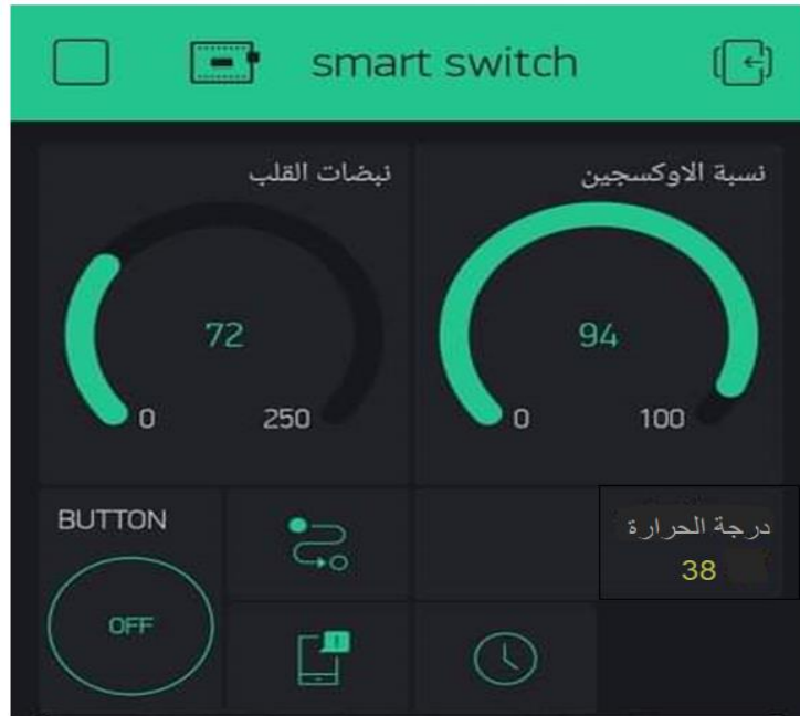
Figure 3. Programming the Blynk application illustrates recording the system in real-time Spo2, pulse rate and body temperature (vital measurements)
