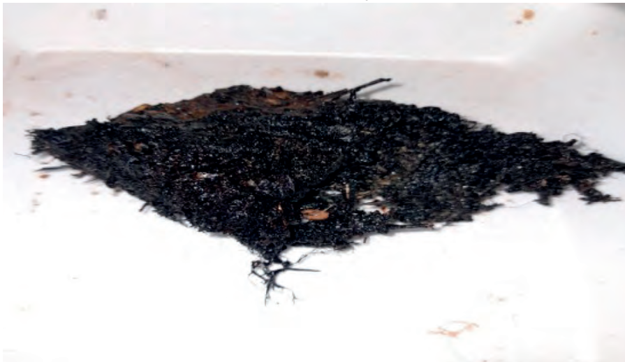
Figure 7. The shape of modified polyurethane foam after immersion in crude oil.
